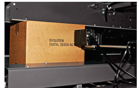
PRINTER MOUNTED IN CARTON SEALER
